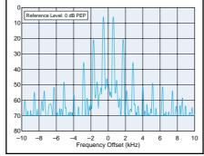
Figure 2—Worst-case VHF/UHF spectral display of the TS-2000 transmitter during two-tone intermodulation distortion (IMD) testing. The worst-case third-order product is approximately 22 dB below PEP output, and the worst-case fifth-order product is down approximately 36 dB. The transceiver was being operated at 100 W PEP output at 50.2 MHz.
