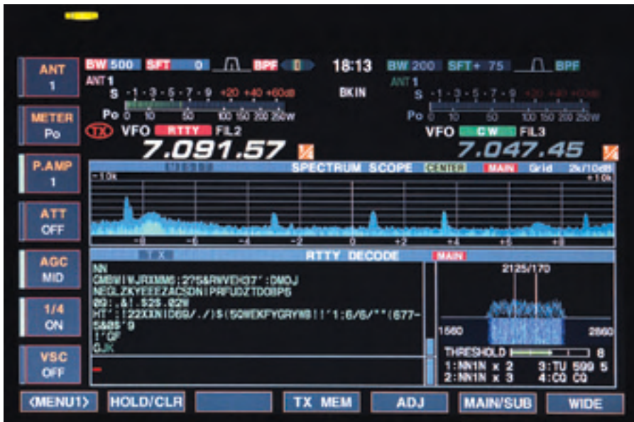
Figure 4 — The IC-7800's RTTY and PSK decoder and tuning indicator make operating digital modes a joy. Just plug in a keyboard and give it a try.
