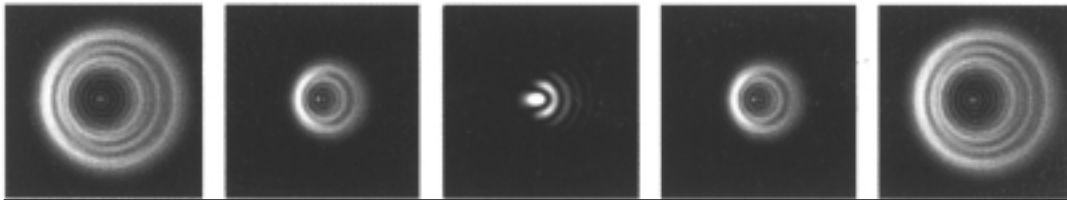
Figure 9-2 -- Even though the star pattern appears the same on both sides of focus, they are asymmetric. The dark obstruction is skewed off to the left side of the diffraction pattern indicating poor collimation.
